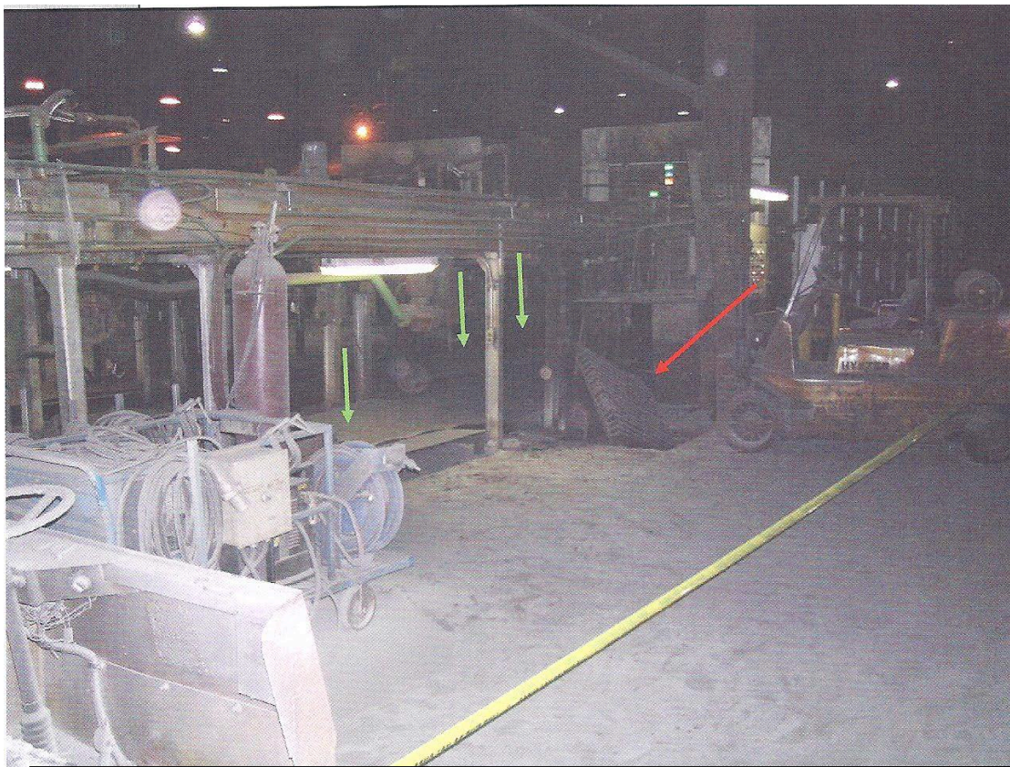
Area where the explosion occurred. Red arrow indicates to the trough cover being removed, Green arrow indicated position of three employees who suffered fatal injuries.
