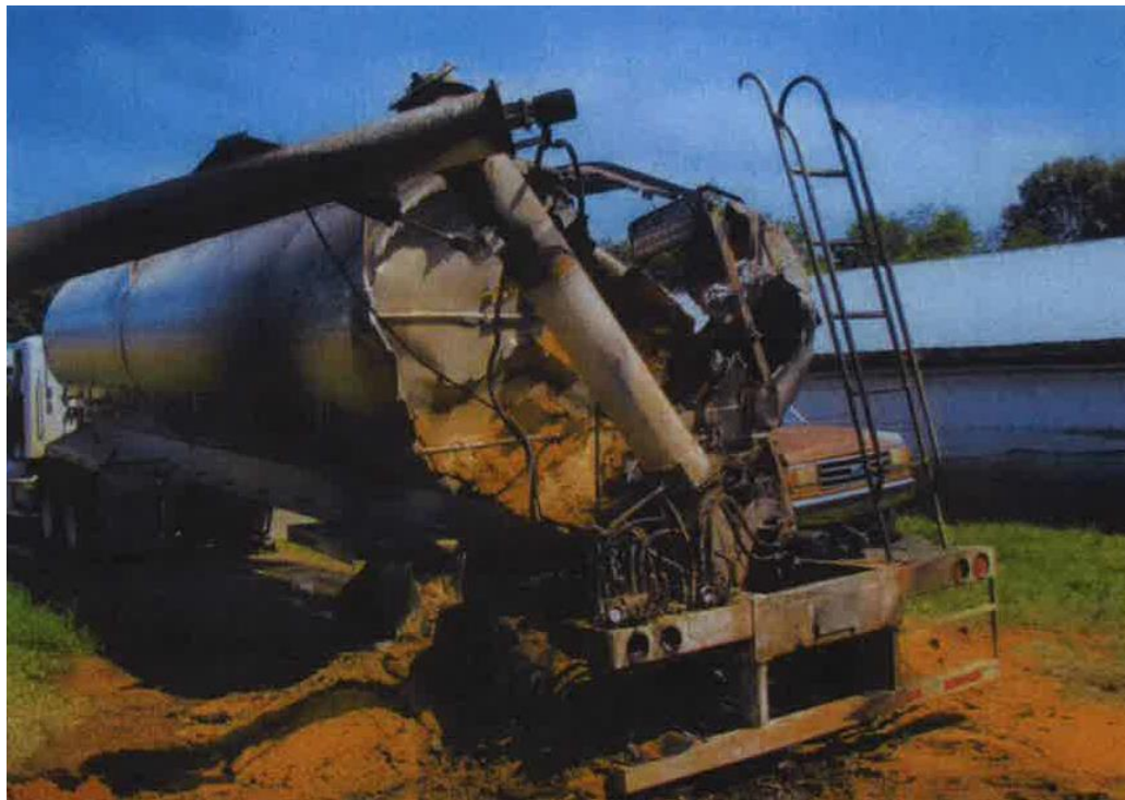
Photo 2 of 2: Truck after stinger contacted overhead power line.
