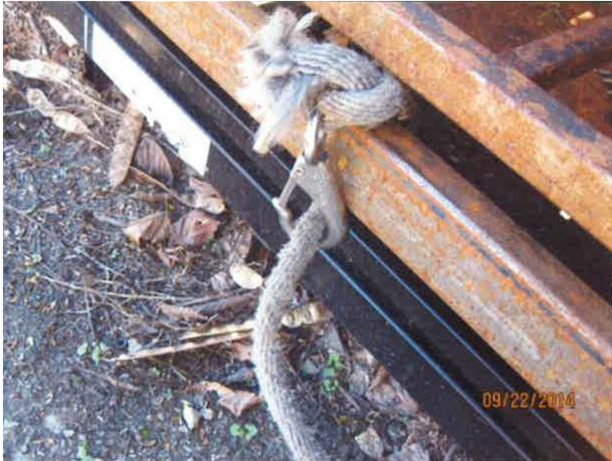
Photo 1 of 1: Manila rope and metal clasp used to pull lawn mowers on metal pallets to the tractor trailer opening for unloading.
