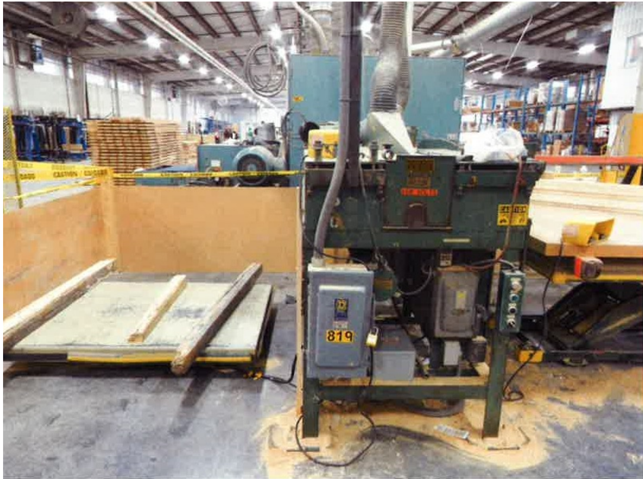
Photo 1 of 2 – Photo of the Lauderdale-Hamilton brand rip saw, and the lifting table located to the left of the saw.
