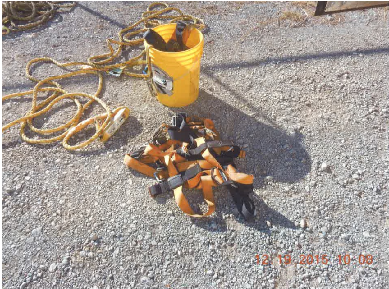
Photo 2 of 2 – Photo shows the fall protection equipment that employees had been wearing but stopped using.
