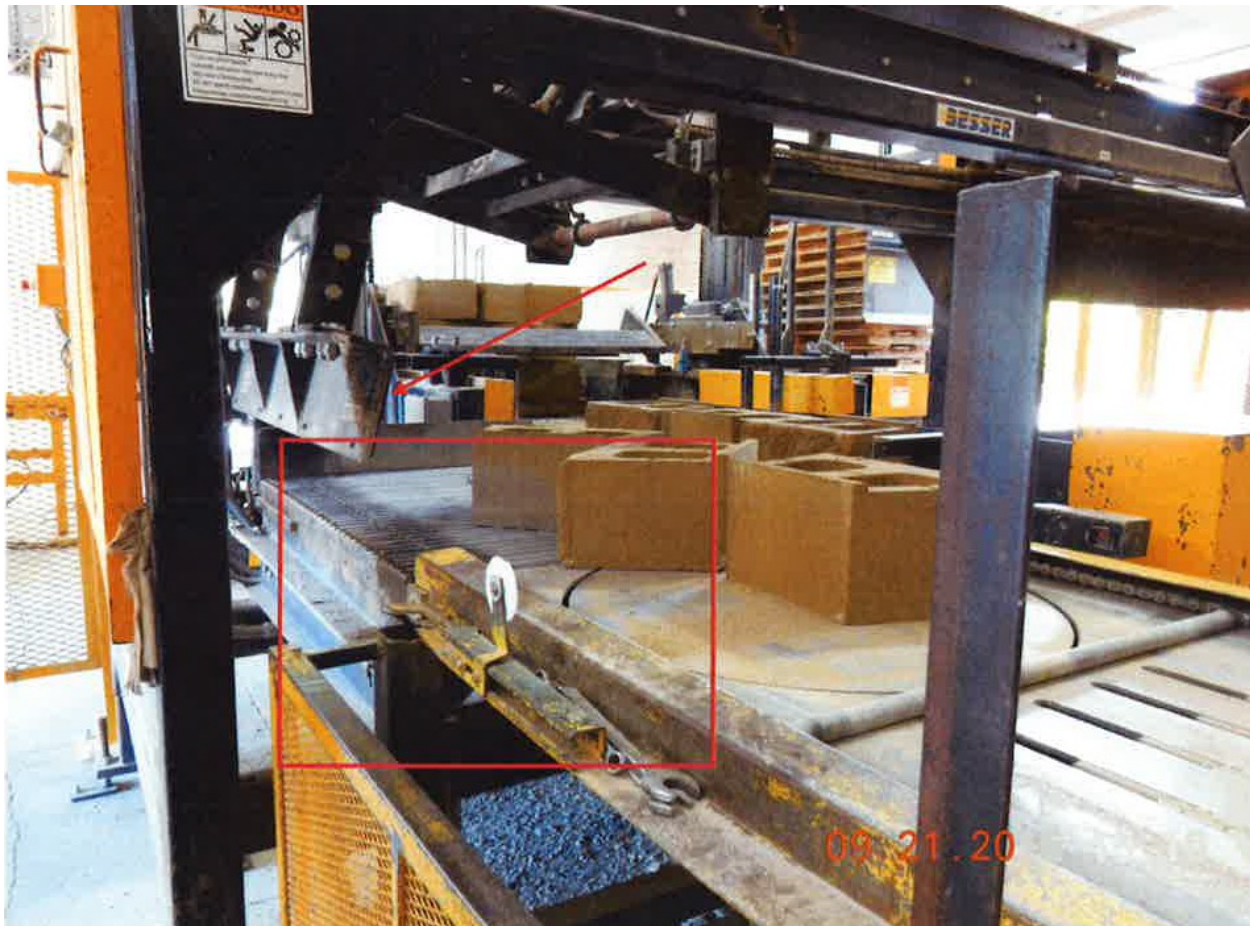
Photo 1 of 1 – The photo shows the overhead side feed area where the victim was found (red square) crushed by the hydraulic arm (red arrow).
