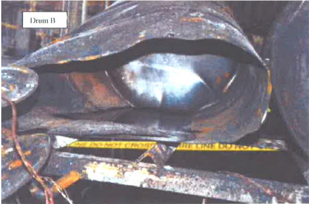
Photo 1 of 1 – Drum B, Category 2 flammable liquid, determined by the Knox County Fire Marshall to be the fuel source of the initial explosion.
