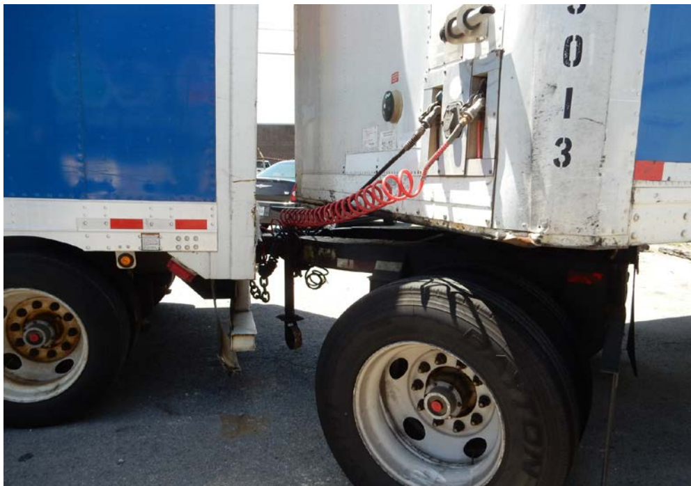
Photo 1 of 1 – Photo shows the area where the victim was attempting to connect the tandem trailers. The victim became pinned between the two trailers when they rolled backward after the trailer brake released.
